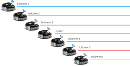
Fig. 2. Illustration of the fixed-time axial alignment tracking problem.
